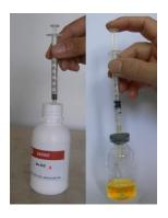
7. Fill the syringe with Reagent 4 to the highest mark (1 ml). Add Reagent 4 by drops until the color become light yellow. Swirl to mix after each drop.
