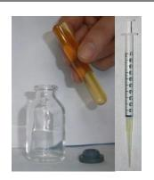
**6.** Fill the titration bottle with one full measuring tube of sample. Attach the yellow tip to the syringe.
