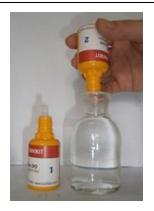
3. Immediately add 4 drops of Reagent 1 and 4 drops of Reagent 2. Stopper the bottle. The sample becomes orange-yellow with a flock.
