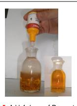
5. Add 4 drops of Reagent 3. Stopper the bottle. Invert the bottle several times. Flock will dissolve and the sample will turn yelloworange if oxygen is present.
