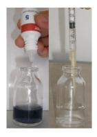
8. Add 1 drops of Reagent 5. Water turns blue or violet. Drop Reagent 4 until colorless end point. Note an used volume of Reagent 4.
